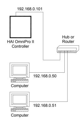
To connect to an OmniPro II controller on a local network using LEVITON PC Access, under *Configure* >> *Network* enter the controller's IP address:
