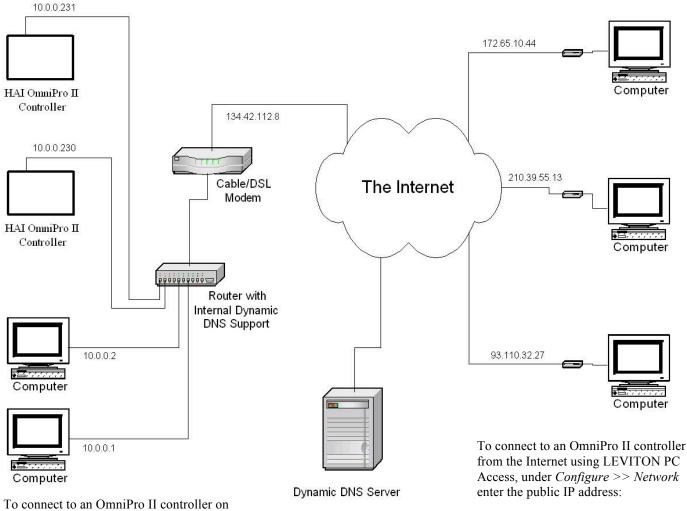
To connect to an OmniPro II controller of a local network using LEVITON PC Access, under *Configure >> Network* enter the controller's IP address:
