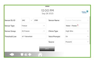
Program the 'Sensor Group', the 'Sensor Name' <sup>1</sup> will follow the associated Water sensor's name plus "- Freeze".
