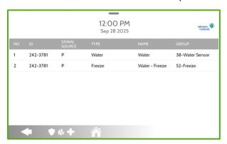
> **Tech Tip:** If the Water zone is deleted, both zones associated with the sensor's serial number will be deleted. The Freeze zone can be deleted if not needed.
