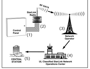
Center; the alarm signals are then forwarded to ANY central station via Contact ID or Sur-Gard System II via TCP/IP using standard line security. The SLE Control Center reports a trouble signal in the event that the network does not receive the expected supervision signal from the wireless communicator. In addition, all models are powered directly from the control panel.
