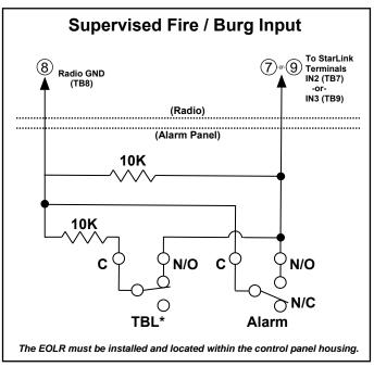
Open = Disarmed Closed = Armed The EOLR must be installed and located within the control panel housing.
