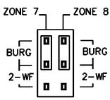
The GEM-P816 can use conventional 12 VDC 4-wire smoke detectors. To use them, select fire zone programming option and do not select 2-wire smoke detector programming option for the desired fire zone (refer to the GEM-P816 Programming Instructions). Set JP3 to the position as shown, if zones 7 or 8 are to be used.
