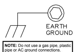
Connect the control panel EARTH GROUND screw to a metal cold-water pipe using at least a #16 AWG. wire. Do not use a gas pipe, plastic pipe or AC ground connections. Also, connect the circuit board to the metal enclosure. Connect a wire with a ground lug crimped or soldered onto one end of the EARTH GROUND screw to the cabinet. **NOTE:** Grounding connections should avoid bends in the grounding wire whenever possible.
