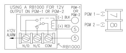
PGM1 and PGM2 are negative switched programmable outputs that can be activated depending on the programming options selected (see GEM-P816 Programming Instructions). Connect the device controlled by the programmable output between terminal 5 (+) and the PGM output (-), either terminal 7 or 8. As an example, the connection to the RB1000 Relay Module is shown.
