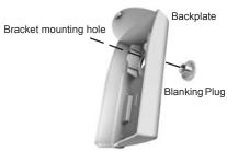
Figure 3. Prep for Wall Mounting (No Bracket)
