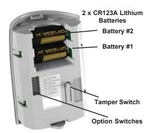
Figure 5. Back View of Sensor
