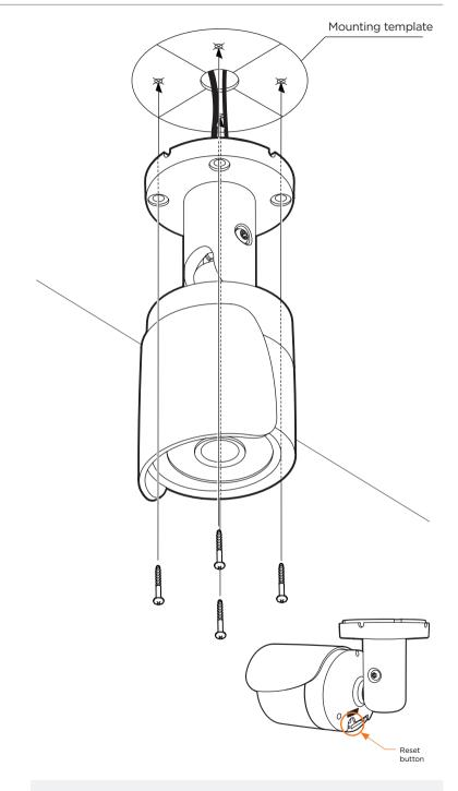
Resetting the camera: To reset the camera, use the tip of a paper clip or a pencil and press the reset button. Pressing the button for five (5) seconds will initiate a camera-wide reset of all the settings, including network settings.
