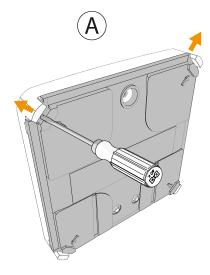
① **Note:** Do not use an electric screwdriver. This causes damage to the plastic enclosure.
